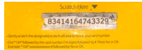
Figure 3: The back of an airtime card used to add airtime to a phone. A user scratches the card to reveal a code, then types in an Unstructured Supplementary Service Data (USSD) number, the # character, and the code. If the code is accepted, the user will get a notification that the account has received a set amount of airtime. If the user wishes to use this airtime to connect to the internet most economically, they enter a second USSD code and select an internet bundle, which provides data that sunsets after a certain amount of time. If the user has enough credit, the bundle will be purchased. A user also checks their account balance via USSD. This interface scales poorly but can be, as in Tanzania, the only one available, making management of a large number of cellular gateways highly labor-intensive.
