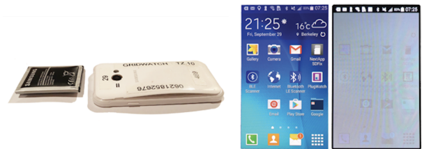
(a) Two swollen batteries.
